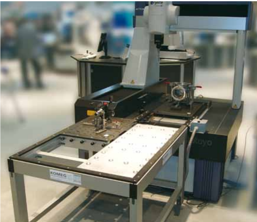
This simplified conveyor accurately positions mass-produced, heavy workpieces on the coordinate measuring machine.
