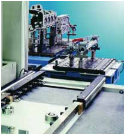
This simplified conveyor accurately positions mass-produced, heavy workpieces on the coordinate measuring machine.
