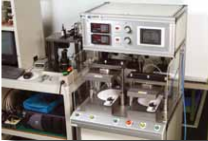
100 % seal integrity test on the production line
