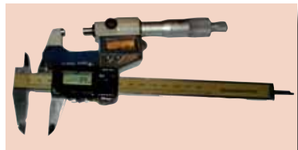
Standard outside micrometer and caliper, "old" design without IP protection.
