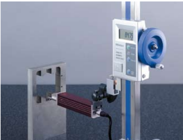
Photo: Measuring a wire-cut surface in orthogonal direction
