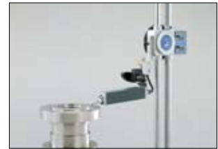
Measurement in the horizontal direction Adapter for height gauge: Code No. 12AAA222
