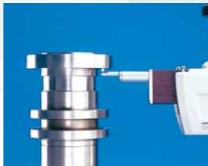
Measurement with probe facing upwards
