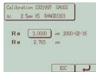
Sample calibration function display
