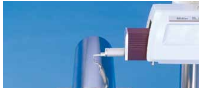
Measuring a cylindrical surface
