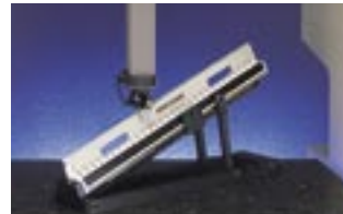
CMM calibration with Check Master No. 515-742
