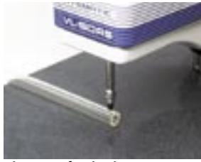
Diameter of resin pipe
